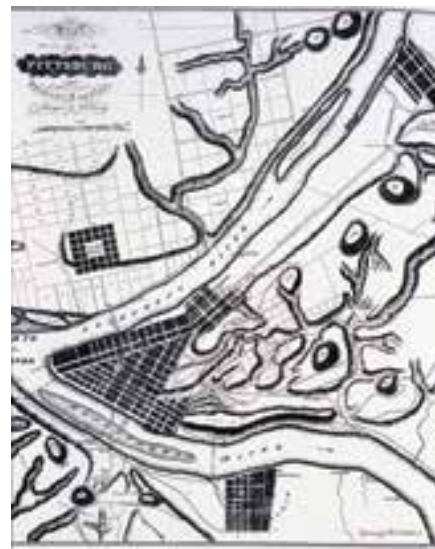
Pittsburg. An early U.S. grid layout responding to different parcels of land. Use of the grid is universal, regardless of size of parcel, orientation of adjacent grid or topography.
