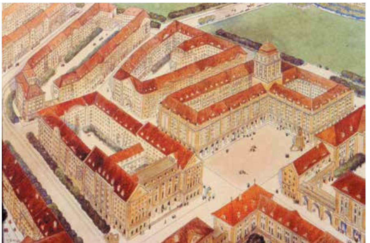
Figure 1: Hermann Jansen, Tempelhofer Feld near Berlin, 1910. The reformed block at scale of the neighborhood: An "architectural square" is combined with a "recreational square"; large uniform blocks with green courts have monumental openings to the public streets.
