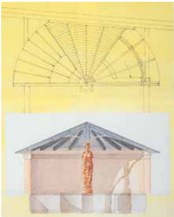
Above: Plan and elevation showing the residential row, L-shaped office building, central garden and underground garages. Drawing: Y. Breithof, Atlante. Left: Pedestrian access pavillion for underground garage with spirial stair and caryatid. Below middle: The 12-story "Blue Tower" undergoing demolition. Photo: Jean-Dominique Burton. Below right: Existing structures before redevelopment. Photo: Gabriele Tagliaventi. Page bottom: Elevation along rue de Laeken. Watercolor by Y. Breithof, Atlante.
